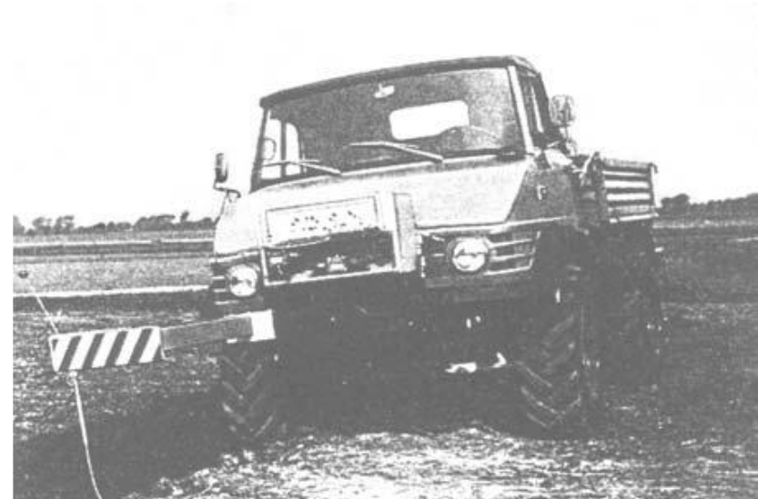
Automated steering (elektro-hydraulic) during plowing, Research by BATEL 1968
