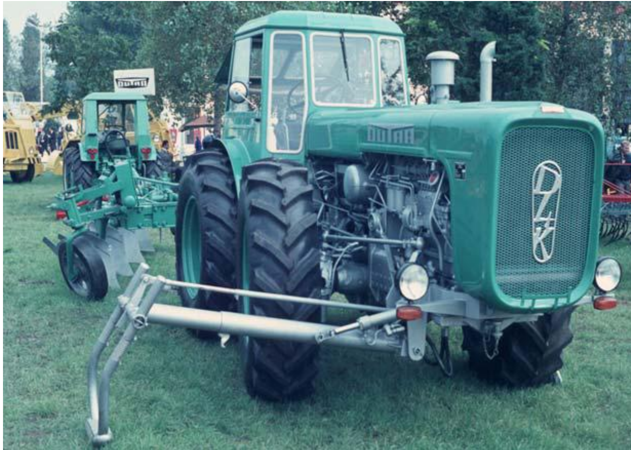
Mechanical guidance along the plow furrow (Hungary)
